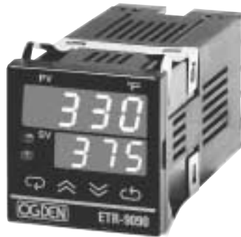
DISPLAY AFTER INPUT SHIFT. ADJUST SV TO 330.
