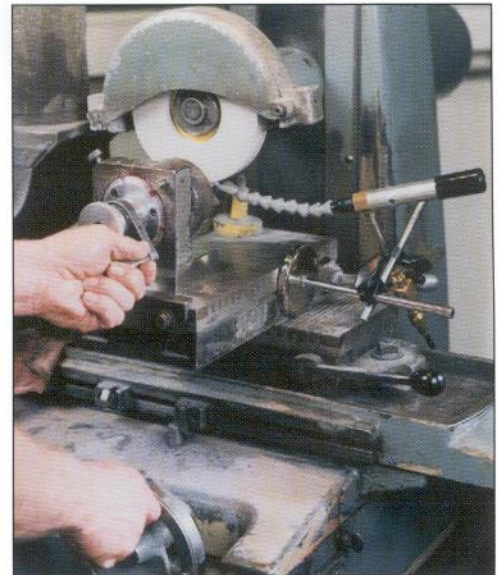
Drastically reduce dry surface grinding production times with the Model 608 Mini Cold Air Gun.
