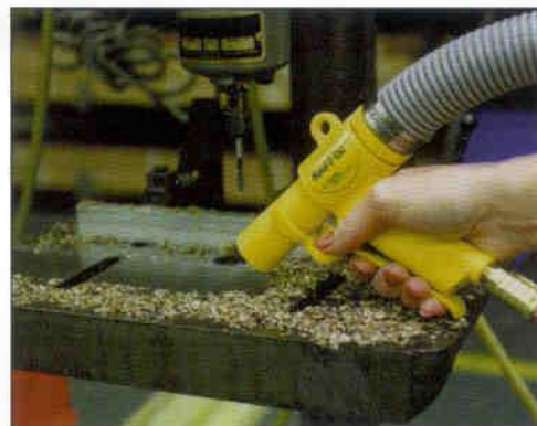
Hand-E-Vac Conveying Kit is ideal for cleaning up metal chips.
