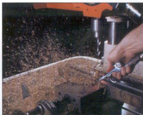
The Model 9401 Blow Gun includes a quiet, air-saving nozzle.
