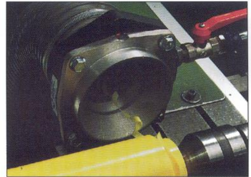
Round Transvectors effectively remove trim and scrap.
